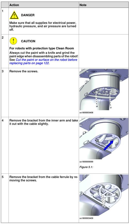
Action Note 1 DANGER Make sure that all supplies for electrical power, hydraulic pressure, and air pressure are turned off. 2 CAUTION For robots with protection type Clean Room Always cut the paint with a knife and grind the paint edge when disassembling parts of the robot! See Cut the paint or surface on the robot before replacing parts on page 122. 3 Remove the screws. 4 Remove the cable ferrule on the cable and take it out. xx1800003410
