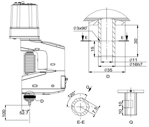
3.3.7 Fitting equipment on the robot (robot dimensions) *Continued*
